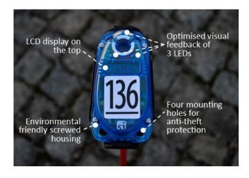
always happen that a runner's hand covered the optical feedback signal. Thanks to the optimised arrangement of 3 LEDs around the hole, the optical feedback signal is now always visible.
